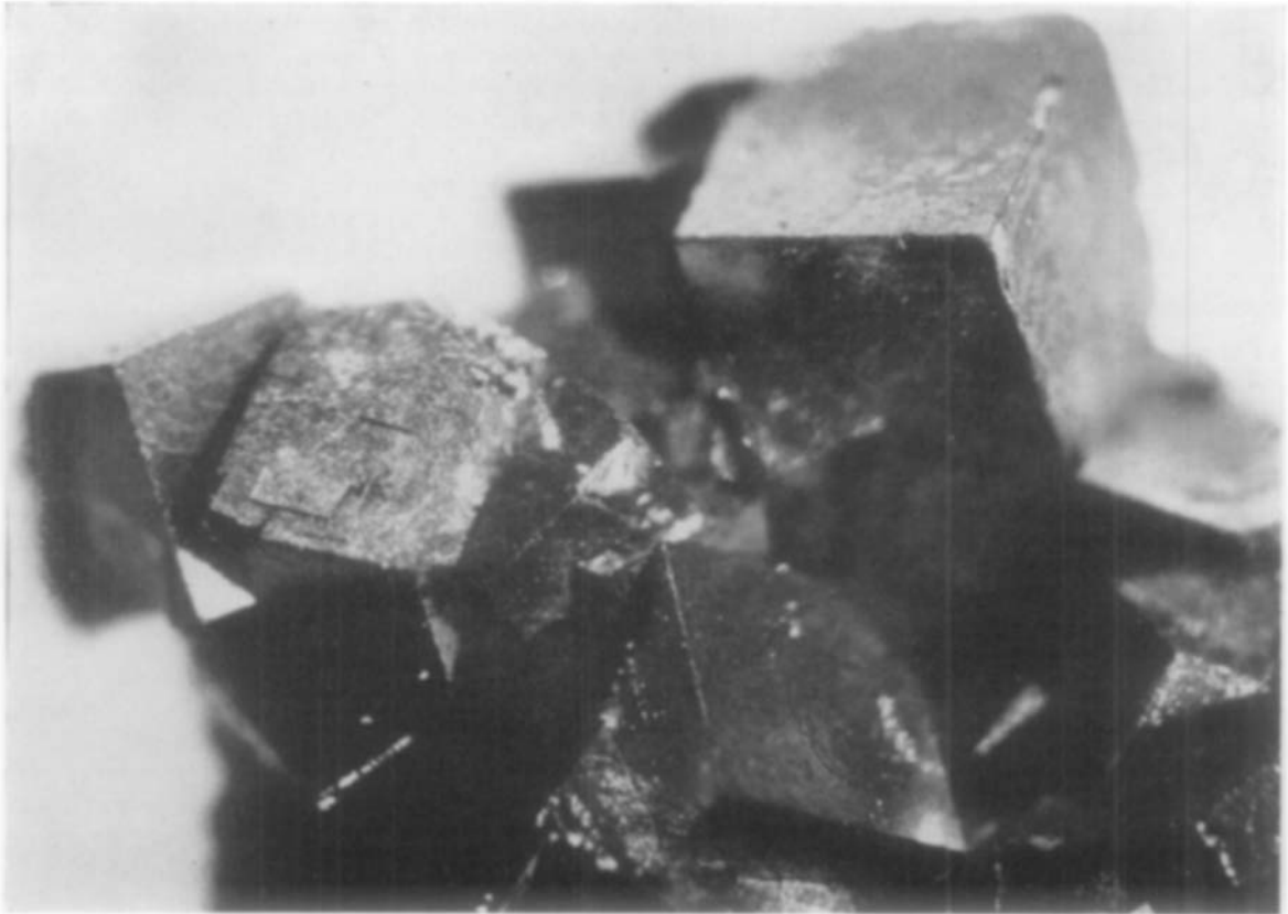
FIG. 1. Typical cubes of Bronze No. 1. Note the steps on some cube faces. Most of these edges are sharp, but some cubes have fissures where cube faces do not quite meet. Magnification 20 (approx.).
